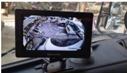
Dedicated fisheye camera and on-board recorder with LCD monitor offer side view to prevent dead-angle on backing a vehicle.
